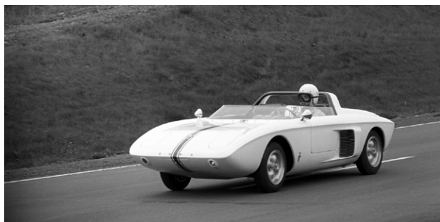
The first Mustang, the 1962 Mustang I, is a two seat, mid-engine sports car.
