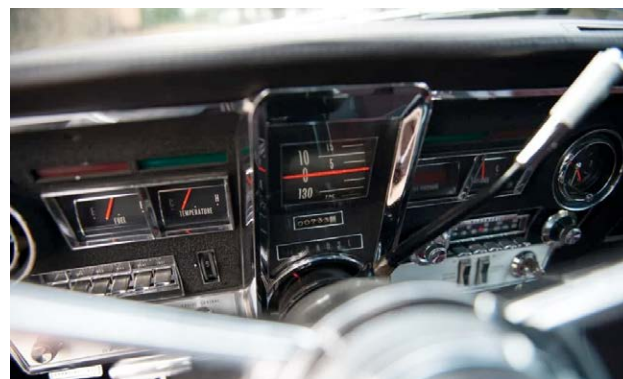
The instrument cluster featured a unique drum speedometer. Photo Credit: RM Sothebys.
