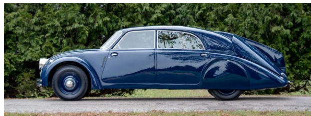
1934 Tatra T77 with its single center-mounted tail fin. Photo Credit: RM Sothebys.
