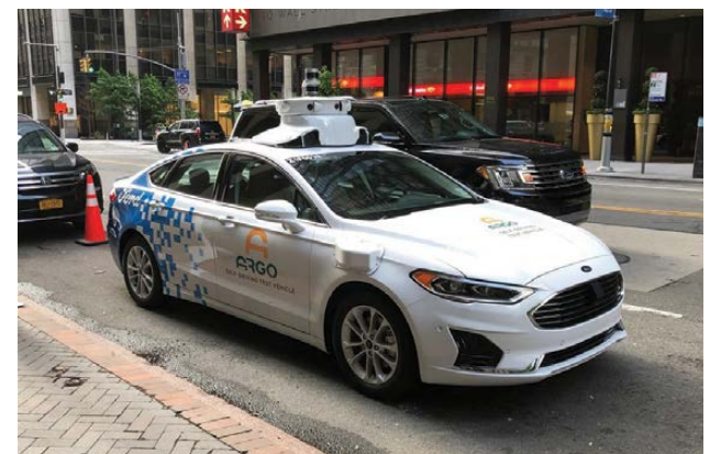
A Ford fusion sedan, modified by Argo AI to operate autonomously, is shown in Manhattan.
