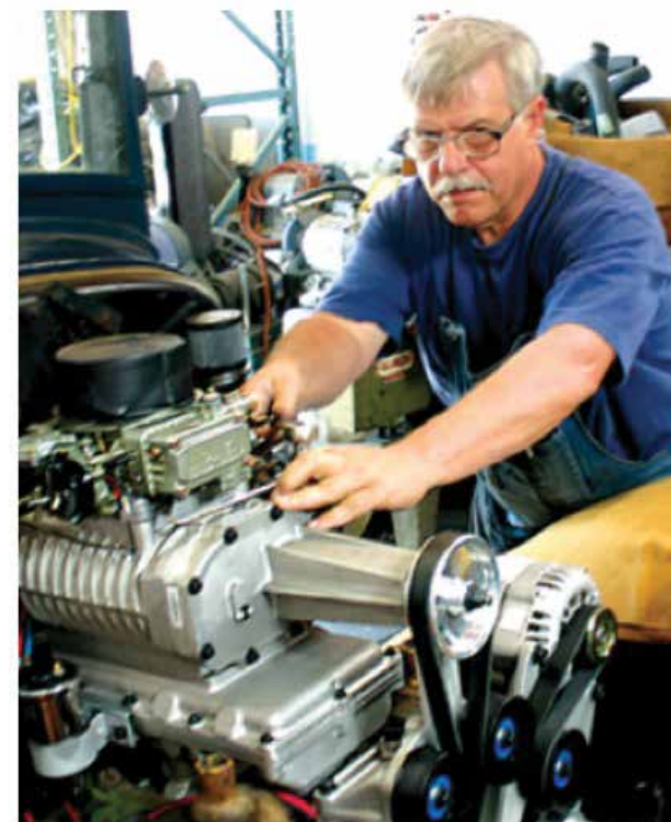
The Tom Roberts/Magnuson Supercharger Kit is designed to be a true bolt-on modification.
